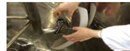
Agitation blade can be removed by hand
