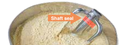
Agitation blade can be removed by hand
